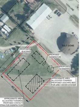
These schematics are a general representative of the preferred alternative. The treatment / storage site would be in proximity to the public works yard and the final location of the components would be determined at detailed design. The raw water lines and watermain distribution system will be developed based on staging of developments and their locations could vary from what is shown. The final municipal well locations will be near the PW2 and TW1-23 sites.
